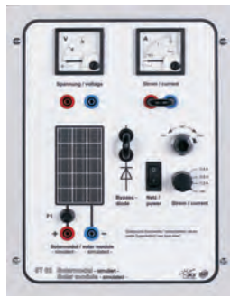
ST 02 Solar Module Simulated
