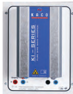
ST 06 S Inverter Island Grid
