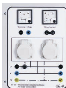
ST 07 AC Load Connection
